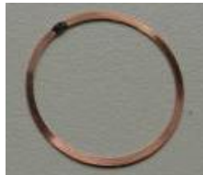
Figure 3 : LF Circular tag
