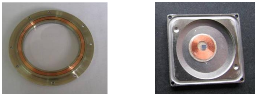
Figure 3. Embedded RF signature in a watch
