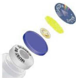
Figure 6: RFID Tag Within Vial Seal
