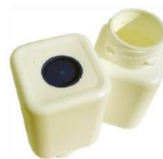
Figure 7: RFID Tag Within Cavity Of Plastic Bottle
